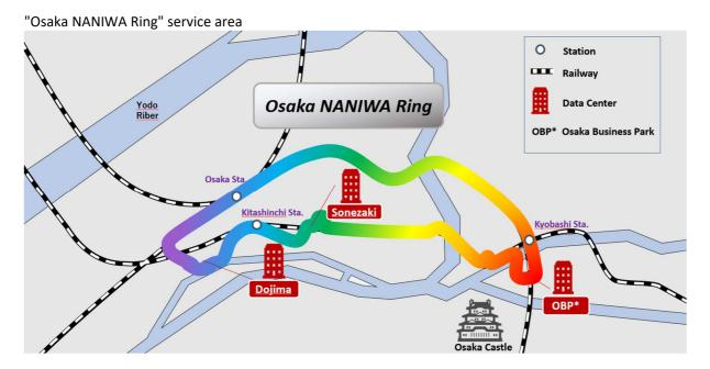
"Osaka NANIWA Ring" is an optical fiber route connecting the newly constructed Osaka Business Park Data Center (location: Kyobashi area, Osaka) with Dojima and Sonezaki, where the major data centers in Osaka are located. The ring leverages JRWON's fiber-optic route for railroads and BBB's fiber-optic knowhow. BBB and JRWON plan to launch the "Osaka NANIWA Ring" in early 2023.
